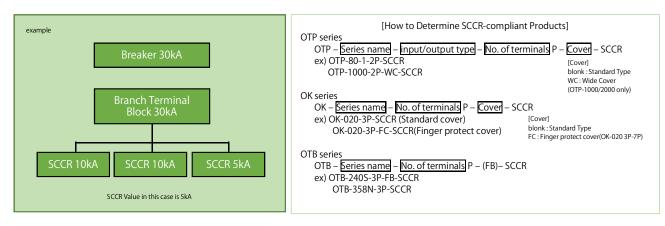
(Attention!) SCCR-compliant products are marked with the SCCR rating. If there is no SCCR marking, the product presents a general purpose terminal block.
